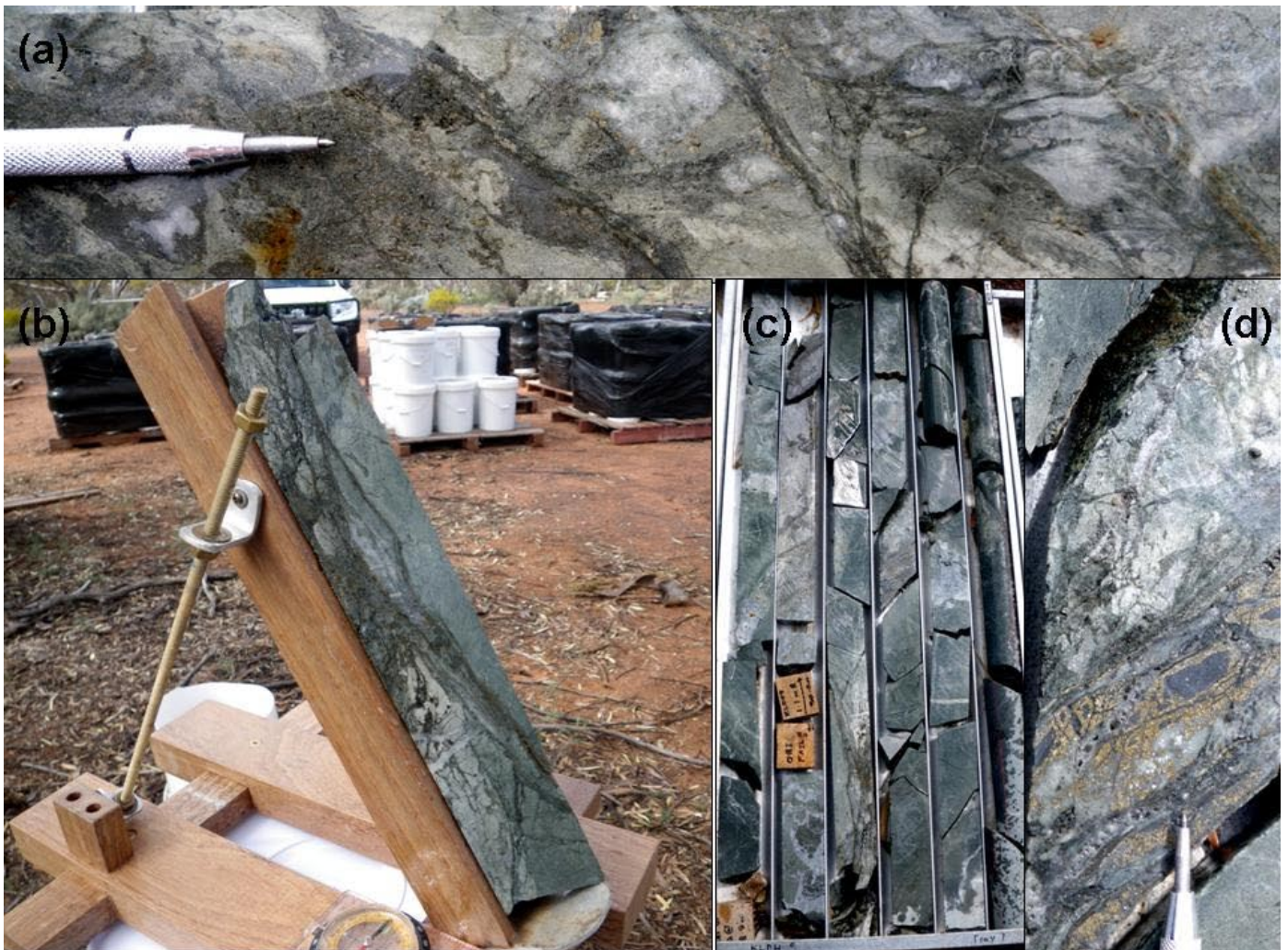
Figure 3: (a) Quartz-carbonate shear vein in basalt with ankerite-silica-albite-pyrite halo, (KLDH09 90m), (b) Ankerite-pyrite-silica-albite shear in basalt dipping moderately southwest (KLDH09, 96m), (c) Domain of shearing and shear veining (KLDH09, Tray 7), (d) Quartz-pyrite-carbonate shear vein with strong ankerite-silica-albite-pyrite alteration (KLDH09, 92m).
